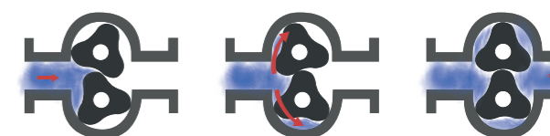
2. Volumetric lobe pump operation
