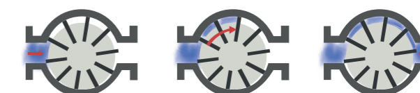
1. Volumetric vane pump operation
